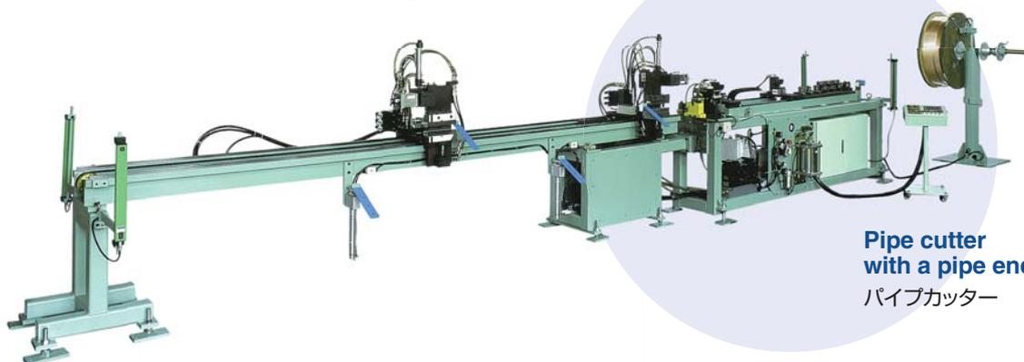
Pipe cutter with a pipe end former
